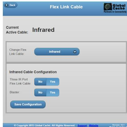
The 3 IR ports on the Tri-port cable can be used as 3 IR emitters (same as the 3 Emitter cable) or 2 emitters and 1 Flex Link Blaster cable on IR3 (same as the 2E1B cable). To use the 2E1B cable, or IR3 of a Tri-port cable with a Flex Link Blaster cable, change the Three IR Port Flex Link cable setting to Yes. Then change the Blaster setting to Yes. For cables with an emitter on IR3 change the Blaster setting to No. Then select Save Changes to apply the new settings.
