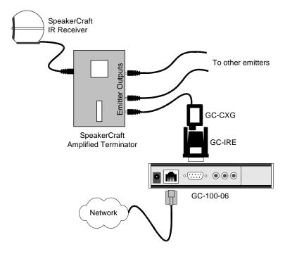
The GC-CXG used with a SpeakerCraft Amplified Terminator and IR Receiver
