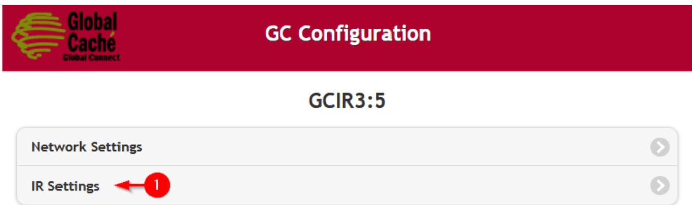
Select IR Emitter, Sensor, Sensor Notify or IR Receiver on each port depending on which cable will be used. If Sensor Notify is selected enter the desired Port and Timer values. Press Apply Changes to save the configuration. All remaining configuration will be done in the chosen control software.
