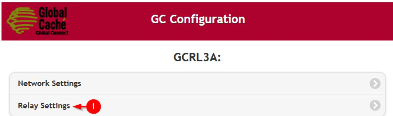
While the GCRL3A module does not require configuration of any relay settings, a testing interface is provided through the web interface for switching the relays. To switch a relay, press the desired ports toggle to turn it On or Off. The relay will change to the set state. All remaining configuration will be done in the chosen control software.
